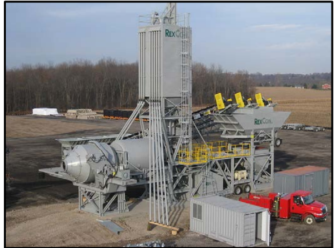
Concrete Batch Plant
